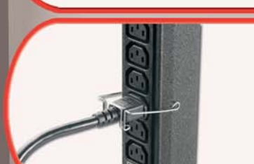
Power Cord Retainers: PRPC13W-2.0-X PRPC13W-2.25-X PRPC19Y-2.0-X PRPC19Y-2.25-X Plug retention devices ensure a secure connection for power cords installed in Panduit Power Outlet Units. For use with Panduit power cords that have IEC 320 C13/C14 and IEC 320 C19/C20 connectors.
